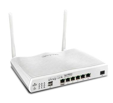
Vigor2866 Series is a dual WAN firewall router. It has one G.fast supported DSL WAN, delivering fiber-like speed up to 1 Gbps, and one configurable Ethernet WAN. The built-in DSL modem is backward compatible with VDSL2 profile 35b supervectoring and ADSL2+. Vigor2866 Series provides load-balancing and failover for your business continuity. Featuring VPN, QoS, route policy, firewall, content filtering, bandwidth management, captive hotspot portal.
