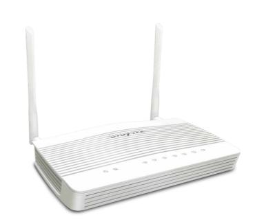
Vigor1100ax is designed for fulfilling FTTH and triple play service demand of fixed network operators or cable operators. The box is based on the mature Gigabit GPON technology, which have high ratio of performance to price. It supports multi WAN connection of bridge or route, IPv4 and IPv6 protocol stack, multicast protocol, QoS and firewall function.
