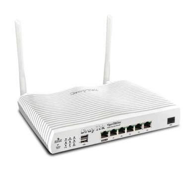
Vigor2865 Series is a VDSL2 35b/ADSL2+ Security Firewall router integrating a DSL modem which is compatible with variants of ADSL and VDSL, including profile 35b supervectoring. There is also a Gigabit Ethernet WAN port for broadband connections to share the traffic load or serve as a failover connection.
