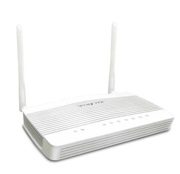
Vigor2767 Series is a VDSL2 35b supervectoring modem, a firewall, and a VPN router. The router has 1x 2.5GbE LAN port which is switchable to be a backup WAN interface. It's highly configurable for an abundance of features including web content filtering, bandwidth limit, QoS and lots more, perfect for professional users who would like to take full control of the network.
