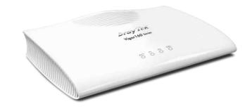
Vigor166 is a G.fast modem/router, delivering fiber-like DSL speed up to 1 Gbps. The built-in DSL modem is backward compatible with VDSL2 profile 35b supervectoring and ADSL2+. With 1 RJ-11 port and 2 GbE LAN ports, It is also configurable to be a small yet powerful router, offering SPI firewall and content filtering by URL keywords and web features.
